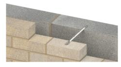
Ties should be selected to provide 62.5mm of embedment in each leaf of masonry to ensure their performance under load. The 2000 Range Tie includes clear embedment markings at 62.5mm to aid with installation. Tie lengths should be selected to provide a design embedment of between 62.5mm and 75mm in each leaf of masonry to ensure their performance under the load as per the table on page 1. The 2000 Range Ties include clear embedment markings at 62.5mm to aid with installation.
