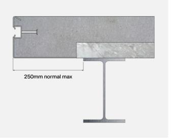
For larger cantilevers it may be necessary to provide temporary propping until such a time as the slab has achieved its required strength.
