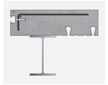
ACS channel must be positioned so that the anchors are positioned within the reinforcement cage to distribute the applied loads back to the surrounding concrete. Local bobs and links are normally sufficient to achieve this, but mesh reinforcement can also be used.
