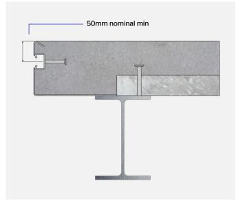
A minimum edge distance of 50mm can be achieved with smaller channel sections. On the larger channel sections the channel must be positioned to ensure that the anchors are positioned within the reinforcement cage.
