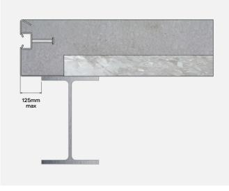
Typically a maximum cantilever of 125mm can be accommodated without the need for temporary propping. However, this is dependent on a range of variables and the ACS Technical Department should be consulted prior to the pouring of concrete. The CET will be supplied complete with stiffening ribs and will require strapping back to the metal deck to prevent overturning of the vertical leg during the casting process.
