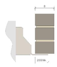
When utilising these, it is important that the shim is fully bearing on the structure to support the compressive forces at the heel of the bracket.
