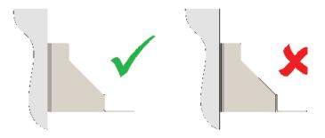
If there is a requirement to introduce a thermal break between the internal structure and Masonry Support system, ACS can provide a 3mm thermal shim as standard. The ACS thermal shim has a thermal conductivity of 0.35W/mK. For more details, please see the technical data sheet for the product.
