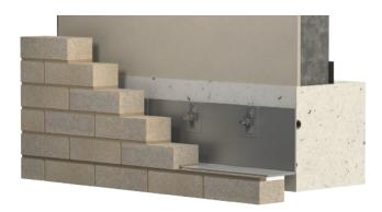
For scenarios where the cavity size is less than 50mm, a T2 system can be utilised. This basic system is used where there is no availability to fit a bracket into the cavity size. Due to the larger bending moment upon the angle at larger cavities, T2 systems become uneconomical and should be replaced with a TI bracket and angle system.
