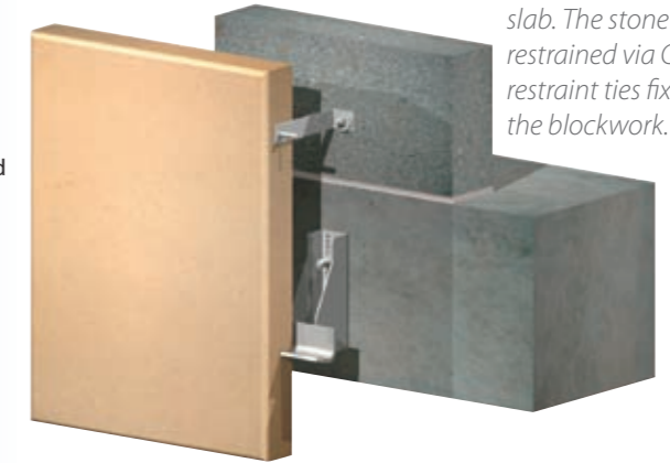
This image illustrates coping stones restrained via C/P/HU restraint ties plugged and screwed to the top of the masonry.
