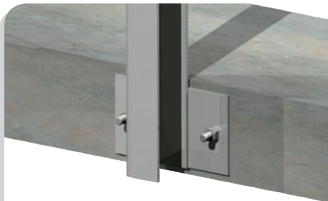
Base connection of an ACS "C" Type windpost fixed to the face of concrete slab using chemical resin studs.
