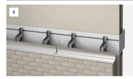
5. Continue to install further pieces of Intex<sup>™</sup> brackets and angle, allowing for around a 10mm gap between units. Each angle should be levelled to the value shown upon the ACS drawings. A string line is commonly used to assist with installation. ACS drawings will show unit references which must be used to ensure the correct pieces are installed.
