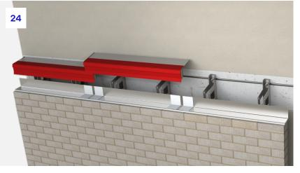
**24.** The next tray can then be placed on top with a minimum of **80mm** overlap between components. Horizontal tolerance in the system is given by sliding the tray along the bracket slot detail.
