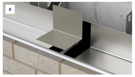
8. Over the top of the joint utilise an Intex<sup>™</sup> jointing piece to bridge the gap. This should overlap each angle by a minimum of 50mm. The piece allows for adjustment either way to allow for site tolerance.
