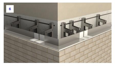
6. Install Intex<sup>™</sup> jointing pieces over all gaps between angles. This requires a double-sided ACS Butyl tape each side of the gap, an Intex<sup>™</sup> jointing piece, and a single-sided ACS Butyl tape for each side of the jointing piece. For further details, please see the main section of the installation guide.
