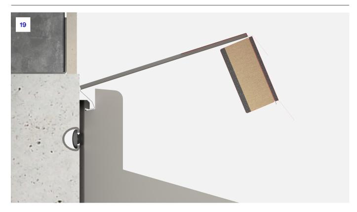
**19.** The tray should be tilted towards the vertical to allow the formed section to sit into the bracket notches.
