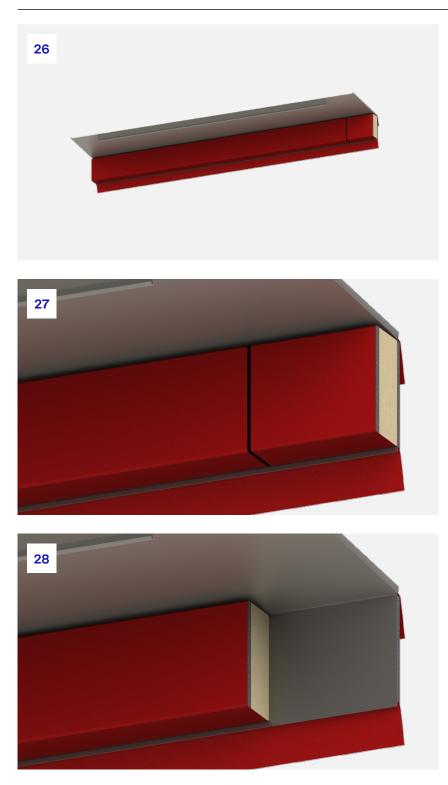
**26.** The mark should be continued around the rear section of the barrier so it is clear where the barrier needs to be cut.
