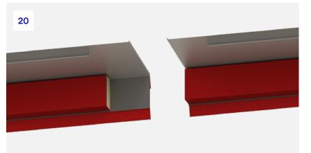
**20.** You will now have a rear barrier with a full end attached to the brackets and an additional cut piece ready for installation.
