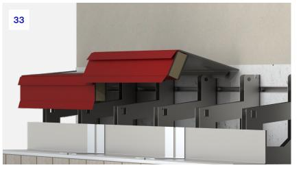
**33.** The bottom lip of the tray section should be pushed fully into the bracket notch to its rearmost face. The bracket notches are specially designed to match the profile of the tray.
