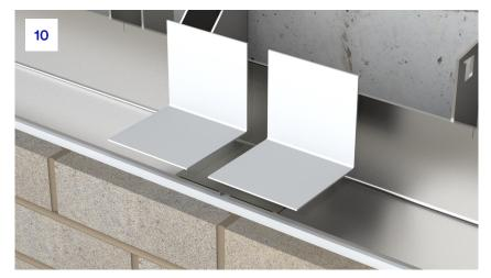
**10.** On top of each side of the jointing piece, a strip of single-sided ACS Butyl tape should be utilised. This should sit half onto the jointing piece and half onto the angle below.
