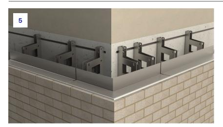
5. Continue to install further pieces of Intex<sup>™</sup> brackets and angle following ACS approval drawings, allowing for around a 10mm gap between units. Each angle should be levelled to the value shown upon the ACS drawings. A string line is commonly used to assist with installation.
