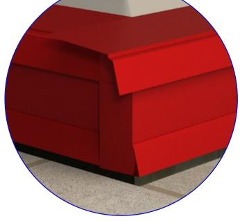
**31.** Brickwork should be built up to the level of the barrier and the wing on the front intumescent strip pushed inbound of the brickwork line. The wings should under no circumstance be built into the brickwork itself. More detail can be seen in the image below.
