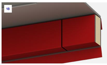
**18.** The mark should be continued around the rear section of the barrier so it is clear where the barrier needs to be cut. By creating a clear mark, this ensures cutting is easy to achieve and reduces the risk of errors.
