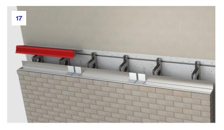
**17.** Once the insulation is in place, it is time to start the installation of the trays. For this section, the insulation has been removed from the images to help with clarity. The relevant first tray should be lined up with the adjoining vertical barrier or structure as per project-specific details. The rear section of the tray should be lined up with the slots in the tops of the brackets.
