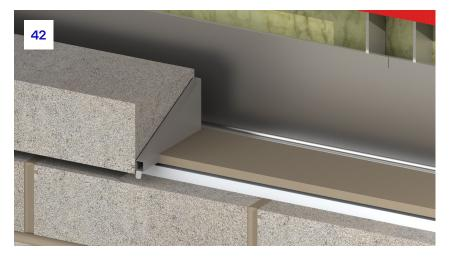
**42.** The system can be used with ACS stainless steel weep vents. These should be used on fresh mortar ensuring any moisture collected on the tray is ejected from the cavity. The lipped section of the weep vent should sit proud of the brickwork to ensure moisture is successfully ejected.
