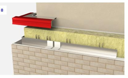
8. Once the insulation is in place, it is time to start the installation of the trays. The corner piece should be installed first and lined up with the brackets located below.
