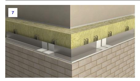
7. Thermal insulation should be tightly installed both between the bracket legs as well as between brackets ensuring it is tight up against all components to create a continuous face for the rear intumescent to expand against. For further details, please see the main section of the installation guide.
