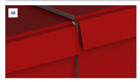
**38.** Once cut, the wing will be free to expand in the case of fire.
