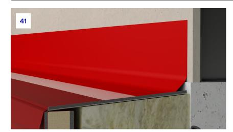
**41.** The membrane/tape should be fully sealed against both the internal structure as well as the Intex<sup>™</sup> top tray as per manufacturer's guidelines.
