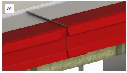
**36.** For both the top and front sections of the tray barrier, the second tray should sit on top of the lower barriers as shown in the image. This ensures continuity in the case of fire.
