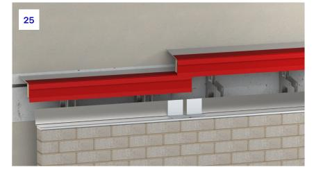
**25.** Once the second barrier is sat on top in the required position, ensuring a minimum overlap of **80mm**, mark the rear barrier where the two barriers meet.
