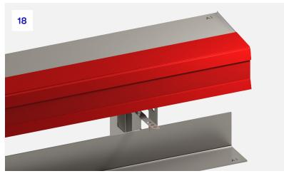
**18.** Each tray has a reference number which will match both the installation drawing, as well as the angle beneath it. This is clearly etched on both the angle as well as the corresponding tray to assist with installation.
