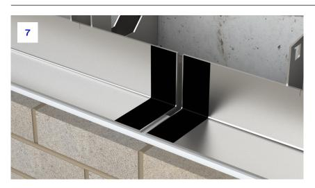
7. Utilise a strip of double-sided ACS Butyl tape on the end of each angle. This tape should be located at the end of the angle and should cover the full height and depth of the section to ensure full coverage against water. The tape has a top covering release layer that should be kept in place at this stage. Ensure that that the tape is fully adhered to the angle. Once in place, the release tape can be removed.
