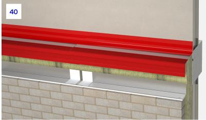
**40.** To allow for typical construction tolerances, a gap is left between the rear of the tray and the internal structure. A membrane or tape should be used to cover this gap, subject to approval from the design team to ensure no moisture can continue down the rear of the façade.
