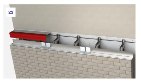
**23.** The tray must be inserted into all brackets along its length to ensure it is fully fixed in place.
