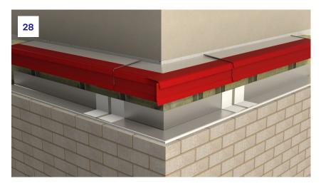
**28.** Once the second tray is in place, the same process can be followed for any remaining trays, ensuring the references match between the drawing, angle, and tray.
