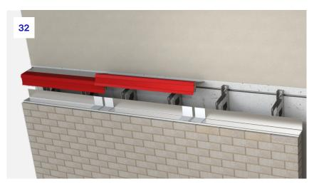
**32.** In the same manner as the first tray, the formed section of the tray can be placed into the bracket notches and rotated into place. See pages 13 and 14 for more details.
