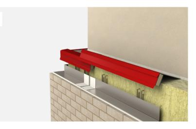
22. In the same manner as the first tray, the formed section of the tray can be placed into the bracket notches and rotated into place. The bottom lip of the tray section should be pushed fully into the bracket notch to its rearmost face. The bracket notches are specially designed to match the profile of the tray. The tray can be fitted around the insulation ensuring a tight fit between all components.
