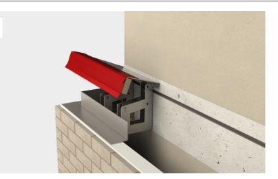
**9.** The right-hand side of the corner tray contains the same formed section as the straight trays to locate within the bracket notches. Each tray has a reference number which will match both the installation drawing, as well as the angle beneath it.
