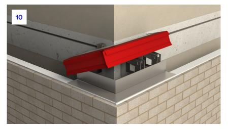
**10.** The tray should be rotated around to allow the formed section to be inserted into the bracket notches. The tray can be temporarily slid to the left to allow for easy rotation.
