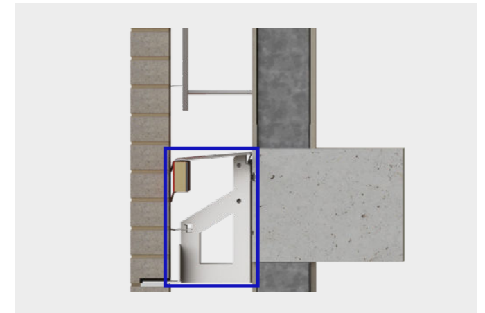
Standard masonry support (top) compared to Intex 4-in-1 Masonry Support system (bottom). Reduces cavity congestion by to 60%.
